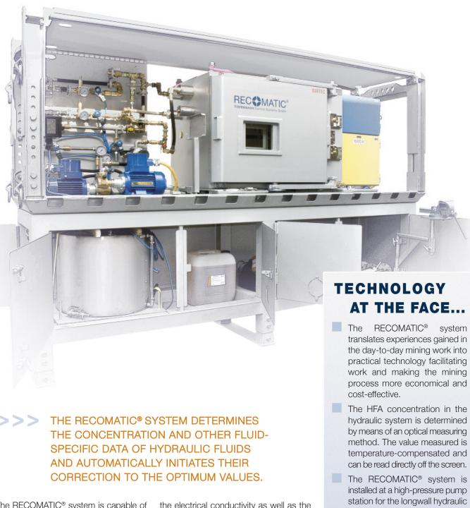
The RECOMATIC® system is capable of regulating the HFA concentration automatically. If the HFA concentration is too low the RECOMATIC® system controls the addition of concentrate via the current measured value. If the concentrate content is too high a water valve opens to dilute the HFA fluid to the set target value.
