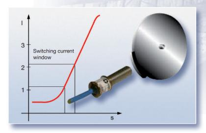
Speed sensing with proximity switches acc. to NAMUR
