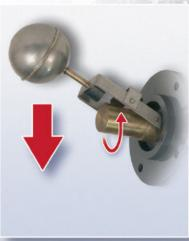
Changing the monitoring function from a rising to a falling fluid level by turning the flange by 180
